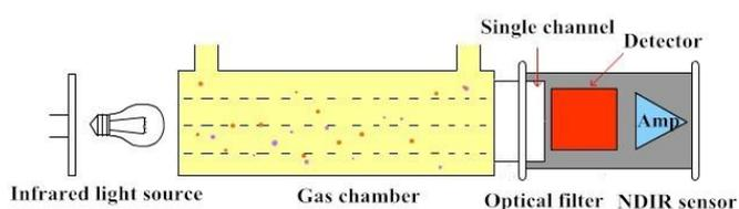
CO<sub>2</sub> molecules inside the gas chamber will only absorb a specific wavelength of the light. The filter allows only the specific wavelength corresponded to pass through it. The detector measures the intensity of infrared light that is related to the intensity of CO<sub>2</sub> and can be described through the Lambert-Beer's Law. The change in sensor signal reflects the change in gas concentration.
