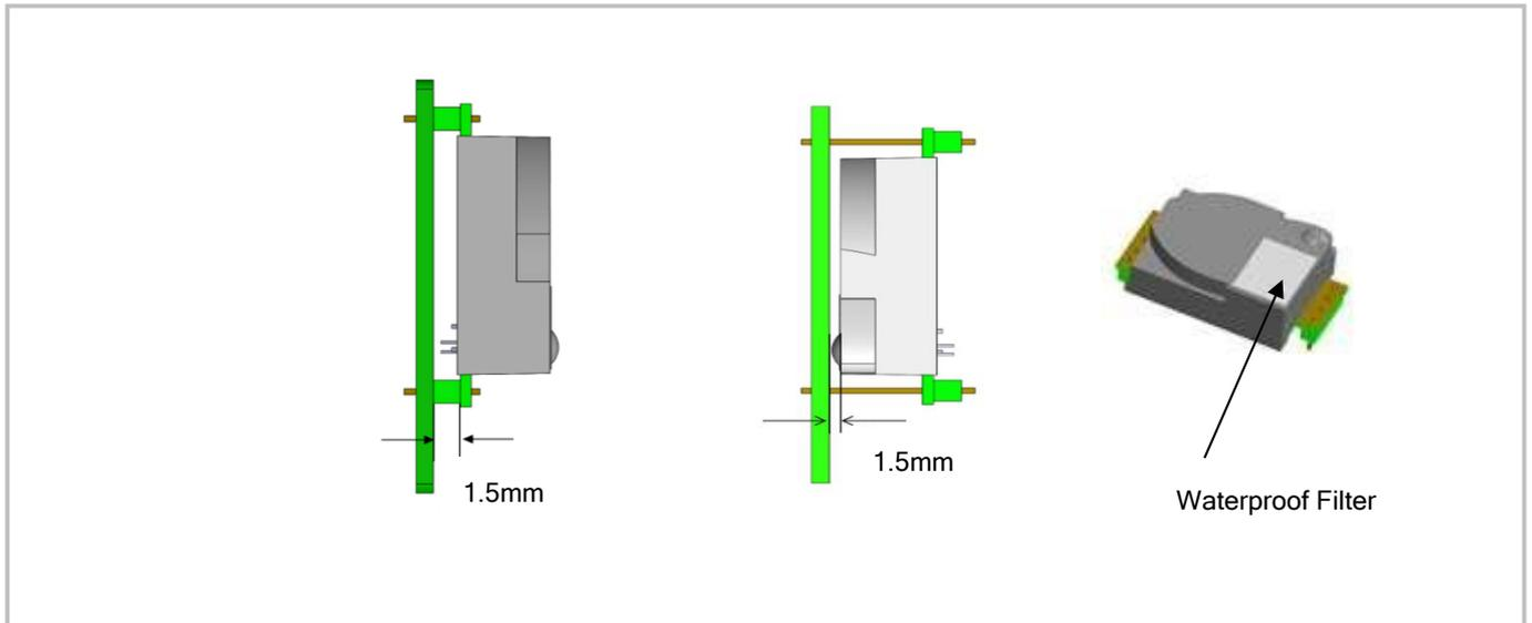
2. To avoid the influence of stress on sensor, please soldering by hand as much as possible when mounting the sensor to the PCB.
