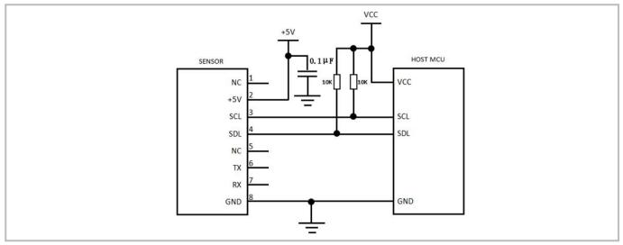
Case 3: 5V-3.3V Level Shift, RX, TX Level Shift
