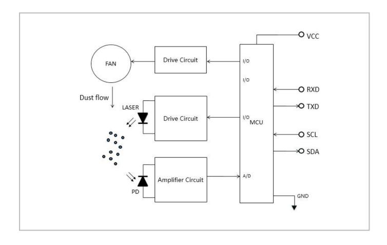
When the fan works, it will generate airflow. When the particles in the sampled gas pass through the beam of the light source (laser), a light scattering phenomenon occurs, and the scattered light is converted into an electrical signal (ie, a pulse) by the photoelectric transformer. The larger the particle size, the larger the amplitude of the pulse signal outputs.
