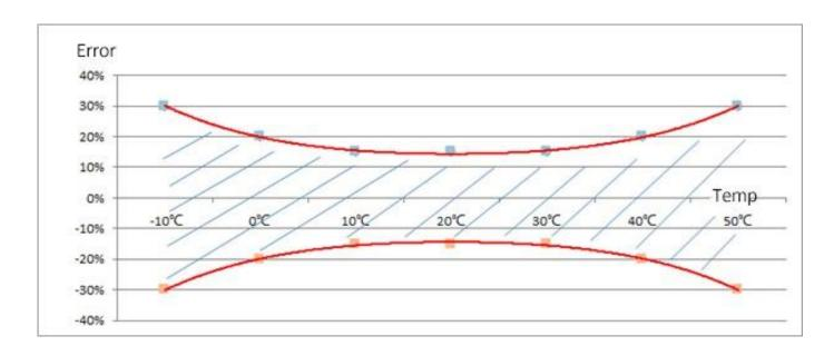
Particle measured error: under  $25\pm2$ °C,  $0\sim1,000\mu$ g/m<sup>3</sup>, consistency and accuracy of PM1.0/PM2.5 is either  $\pm15\%$  reading or  $\pm15\mu$ g/m<sup>3</sup>, the bigger one is considered.
