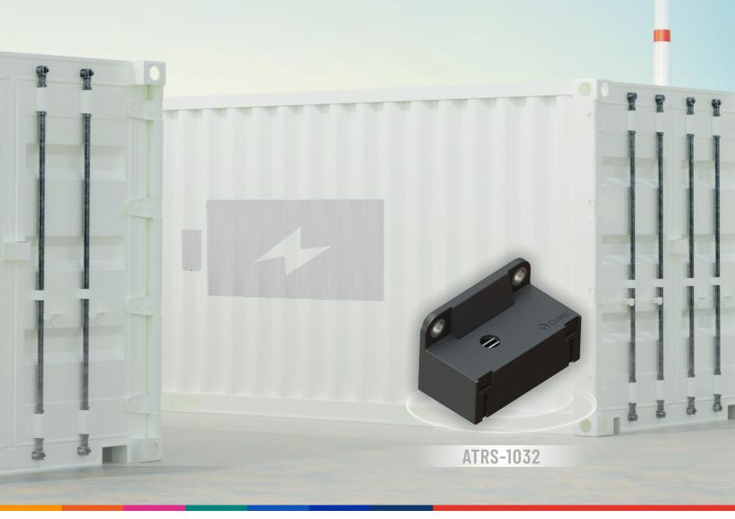
Cubic ATRS-1032 is a lithium-ion battery thermal runaway monitoring sensor based on light scattering and MEMS thermal conductivity (TC) technologies. The ATRS-1032 is specifically designed to effectively monitor the concentration of particulate matter and H2 released during the early stages of thermal runaway while transmitting warning signals to the battery management system (BMS).
